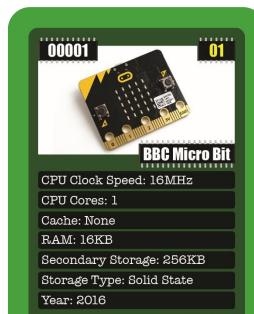
Featuring an accelerometer, a 25 LED display and Bluetooth connectivity. The Micro Bit can be programmed using blocks or Python. This tiny computer has been used to make wearables, bike lights and even a weather station.
